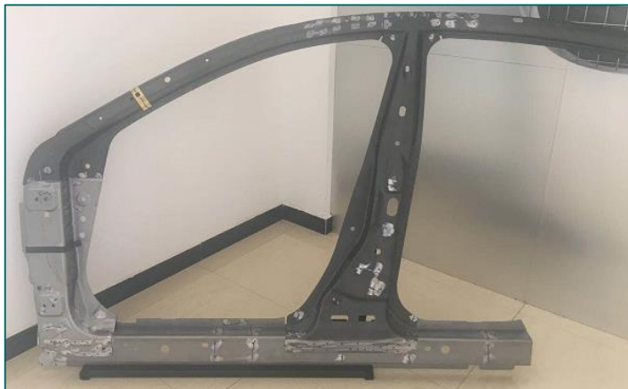
B/S Reinforcement Plate Welding Assembly
