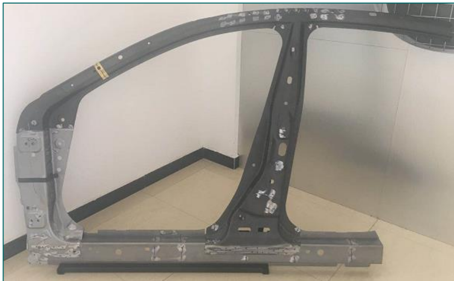
B/S Reinforcement Plate Welding Assembly
