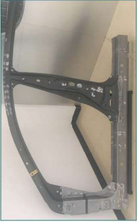
B/S Reinforcement Plate Welding Assembly
